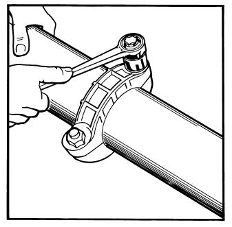
Fig. 15 — Installed Coupling Fastening Grooved Pipe Ends
